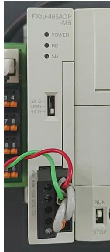
**II. Connect the COM (RS485 A/B) on the left side of the FX3U to the interface module (1/2) to convert it to a RJ45 connector before connecting it to the main controller**
